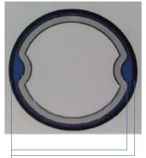
2 bigger air gaps makes airflow easier with result of low head los
